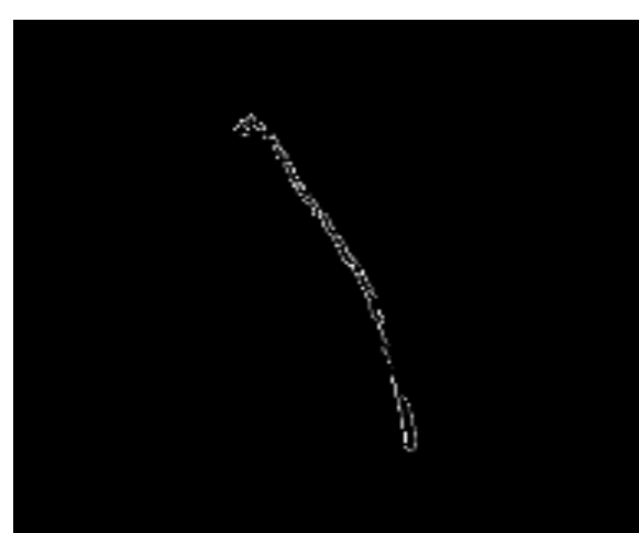
Streak after Gaussian blur and edge detection.
