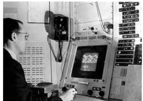
"When there was only one personal computer... " The UR-Vision: Ivan Sutherland and Sketchpad on TX-2 3am-6am at Lincoln Labs in 1962
